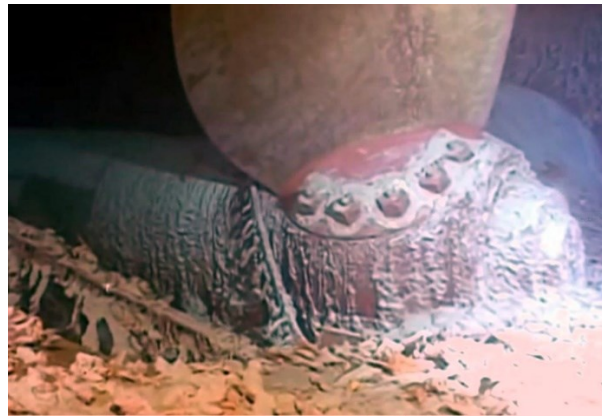
Antifouling paint remnant of Titanic propeller
