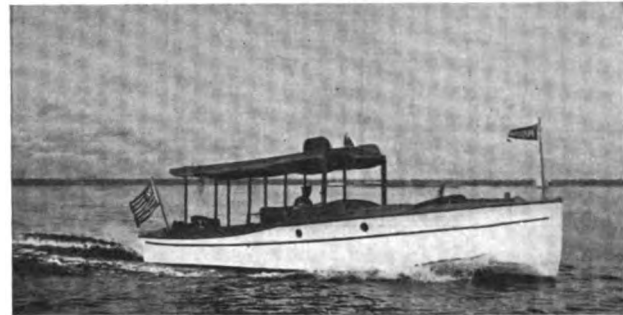
A 30-Ft. Hand V-Bottom Cruiser, Powered with a 40-H.P. Loew-Victor Engine. Speed 15½ M.P.H.
